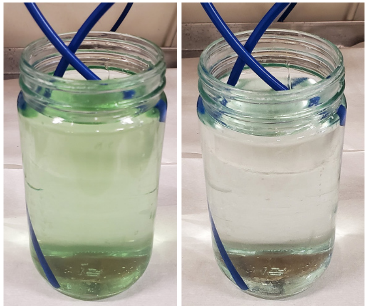
Before: “Raw” wastewater contained 701 ppm copper.
